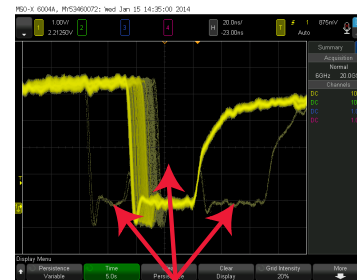
Infrequent glitches and signal jitter captured after one second on 6000 X-Series with standard update rate.
